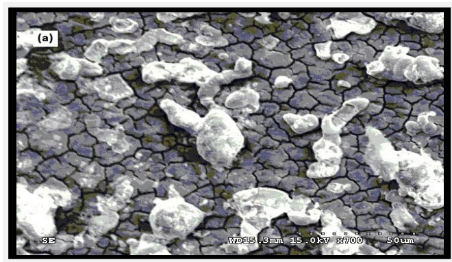
Figure S2. SEM micrograph of the chrome steel ball surfaces after immersion of 72 h in the presence of 0.1 mM 2-(2-hydroxybenzylideneamino)phenol in 0.1 N HNO 3 .
